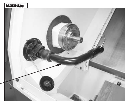
SHOWN WITH TOOL PROBE INSTALLED
