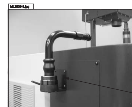
LEFT SIDE OF MACHINE TOOL PROBE SHOWN WHEN NOT IN USE
