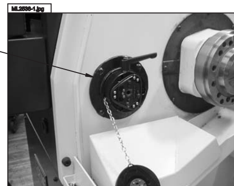
CAP OFF WITH TOOL PROBE REMOVED
