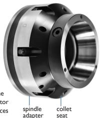
Reduce the clamping pressure of the machine to a minimum and extend the drawbar to the forward position. Carefully screw the clamping sleeve #2 onto the drawbar clockwise until it bottoms out. DO NOT TIGHTEN. Align the key in the collet seat with the keyway in the clamping sleeve to push the collet seat onto the spindle adapter. Rotate the body
